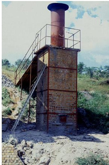
Figure 2: An improved vertical shaft kiln in Zimbabwe. Photo: Kelvin Mason / Practical Action.
